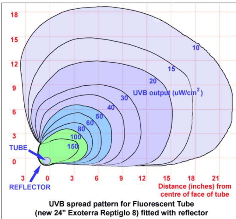
This is the spread chart for the same tube when fitted with a reflector. As expected, the reflector throws the light from the back of the tube forwards and creates a more intense beam of UVB light. The output of the tube is "shaped" into a flattened cylinder which puts useful UVB considerably further into the vivarium.
