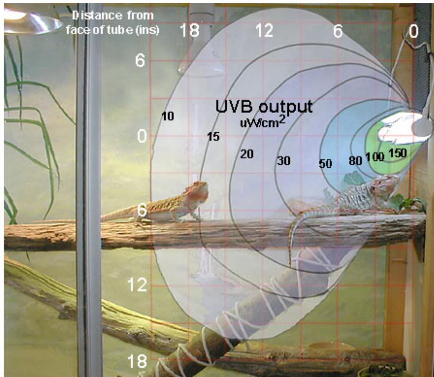
**A visualisation of a typical UVB spread pattern for a Fluorescent Tube fitted with a reflector, in the vivarium.**
