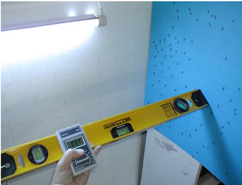
In the photograph you can see a reading of  $37\text{uW}/\text{cm}^2$  on the meter. This picture was taken while I was mapping the  $40\text{uW}/\text{cm}^2$  range... in this case I'd need to move the meter fractionally closer to the tube, whereupon the meter would read 40 and I would mark the chart at the corresponding point.
