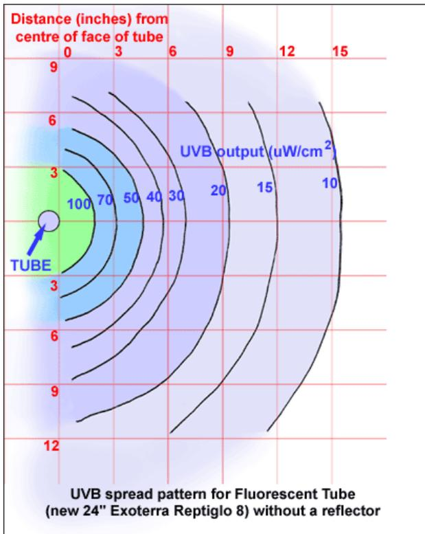
This is the spread chart for the fluorescent tube without a reflector. The black lines are those which connect my measured data points; the coloured zones are extended purely to help visualise the pattern which could be seen.
